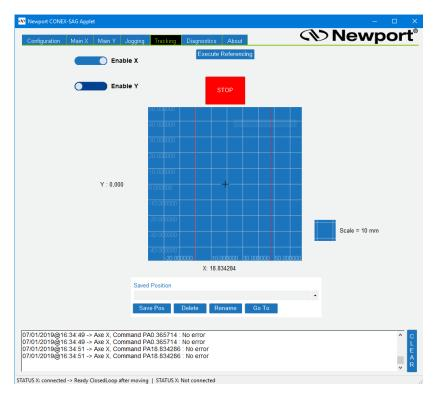
Choose the position desired with the mouse and click. The stage displace to the position.
