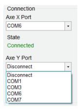
• In case a wrong port is selected, after searching for some time, the "Not connected" state is displayed and an error is reported in the communication area.
