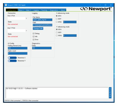
• The communication area in the bottom displays the commands and errors. This area appears in all the different tabs. It can be erased with the "Clear" button on the right.
